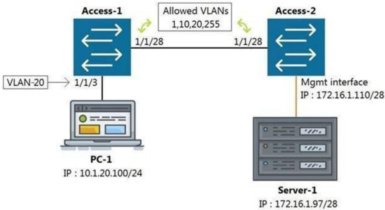
All switches are running Aruba OS-CX. While working in the terminal of Access-2, you are unable to reach Server-1 using SSH. What is the correct command to ping Server-1 from Access-2 to test reachability?
