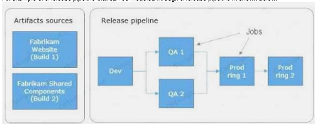
In this example, a release of a website is created by collecting specific versions of two builds (artifacts), each from a different build pipeline. The release is first deployed to a Dev stage and then forked to two QA stages in parallel. If the deployment succeeds in both the QA stages, the release is deployed to Prod ring 1 and then to Prod ring 2. Each production ring represents multiple instances of the same website deployed at various locations around the globe.
