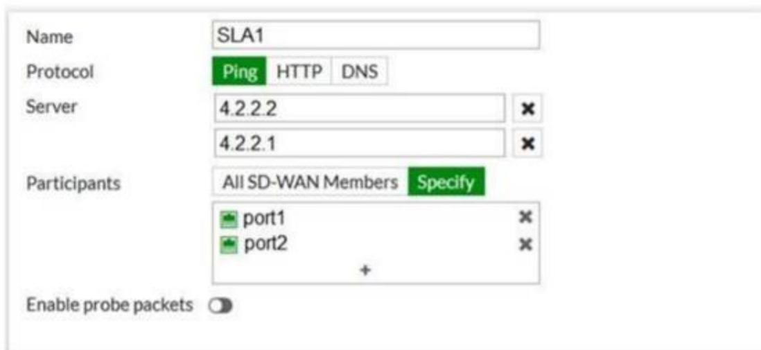
An administrator has configured a performance SLA on FortiGate, which failed to generate any traffic. Why is FortiGate not sending probes to 4.2.2.2 and 4.2.2.1 servers? (Choose two.)
