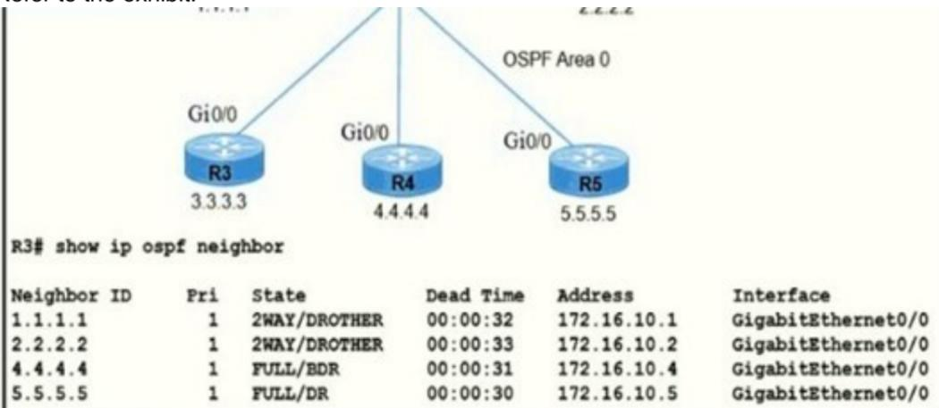
R5 is the current DR on the network, and R4 is the BDR. Their interfaces are flapping, so a network engineer wants the OSPF network to elect a different DR and BDR. Which set of configurations must the engineer implement?
