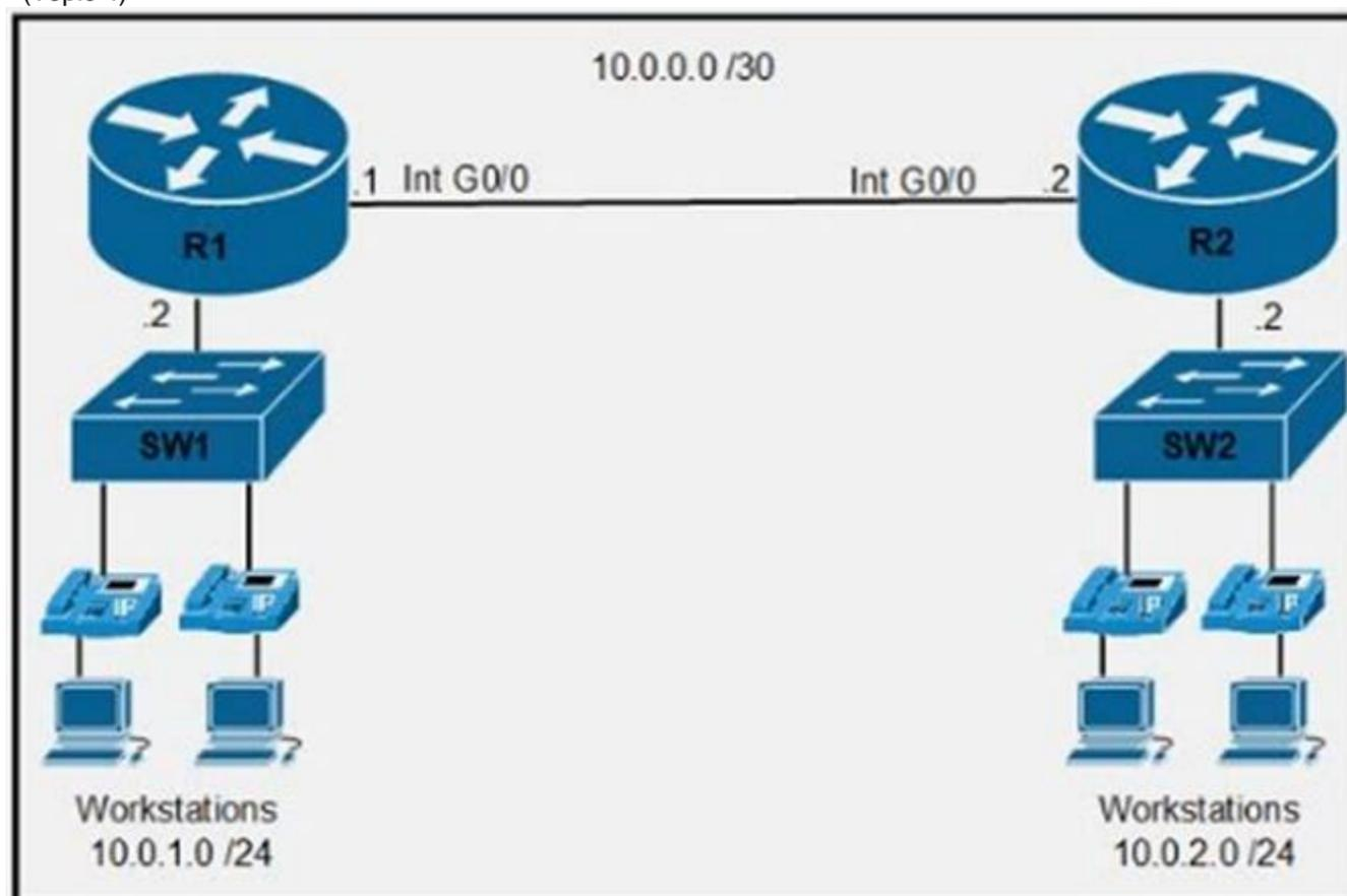
Refer to the exhibit. An engineer is asked to configure router R1 so that it forms an OSPF single-area neighbor relationship with R2. Which command sequence must be implemented to configure the router?
