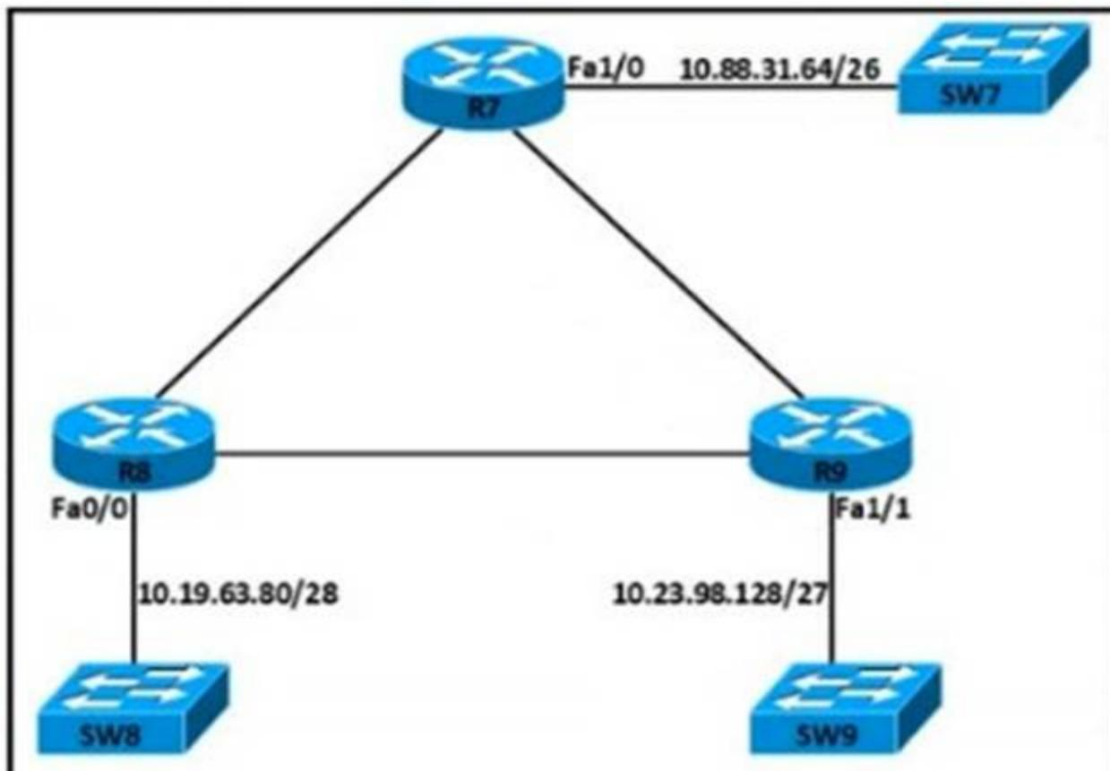
Refer to the exhibit. Each router must be configured with the last usable IP address in the subnet. Which configuration fulfills this requirement?
