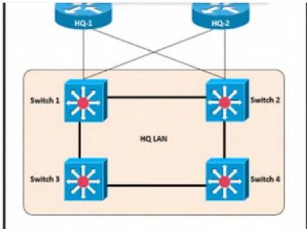
After the election process what is the root bridge in the HQ LAN?
