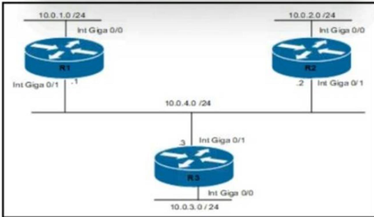
Routers R1 and R3 have the default configuration The router R2 priority is set to 99 Which commands on R3 configure it as the DR in the 10.0 4.0/24 network?
