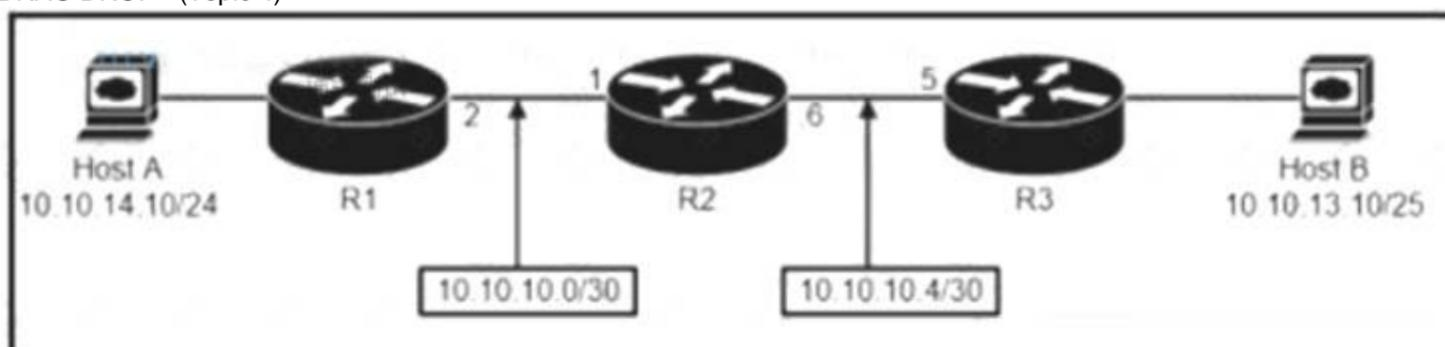
Refer to the exhibit. An engineer must configure a static network route between two networks so that host A communicates with host B. Drag and drop the commands from the left onto the routers where they must be configured on the right. Not all commands are used.
