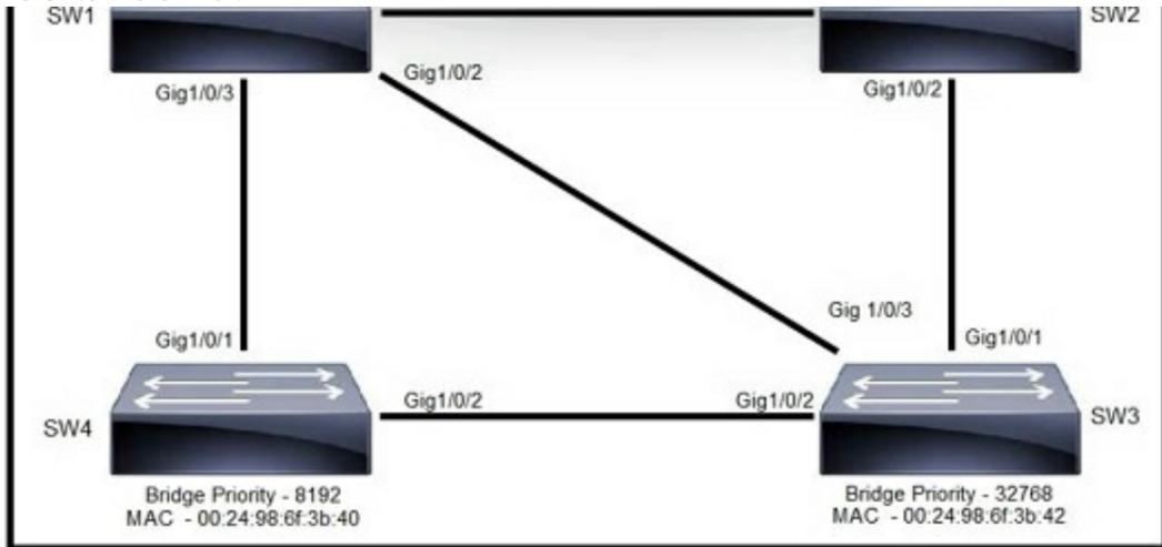
Rapid PVST+ mode is on the same VLAN on each switch. Which switch becomes the root bridge and why?
