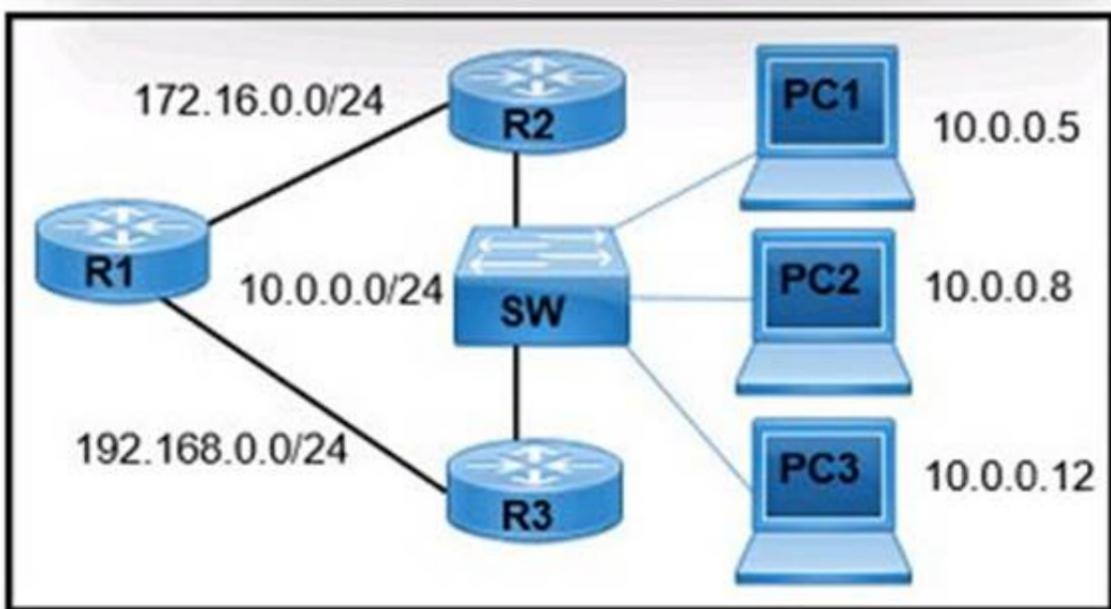
A network engineer must configure R1 so that it sends all packets destined to the 10.0.0.0/24 network to R3, and all packets destined to PC1 to R2. Which configuration must the engineer implement?
