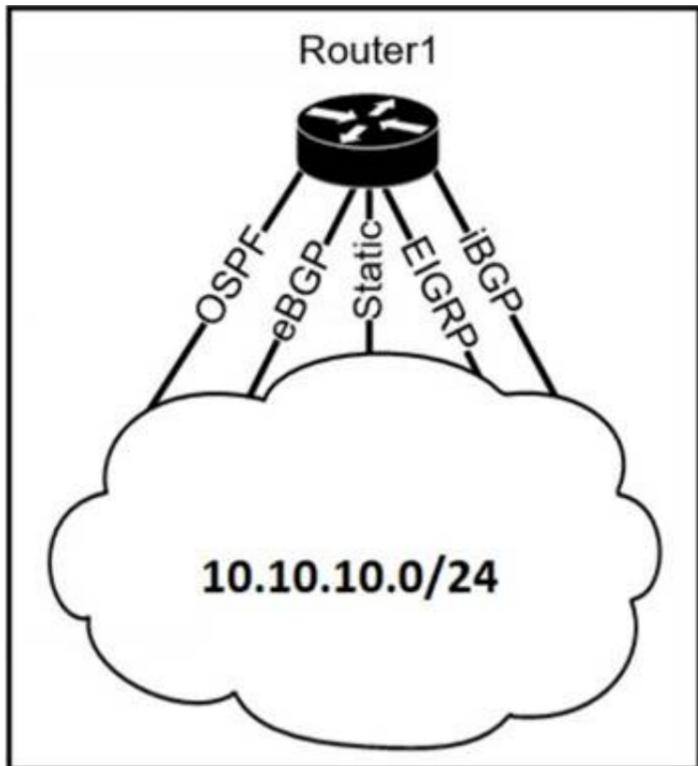
The Router1 routing table has multiple methods to reach 10.10.10.0/24 as shown. The default Administrative Distance is used. Drag and drop the network conditions from the left onto the routing methods that Router1 uses on the right.
