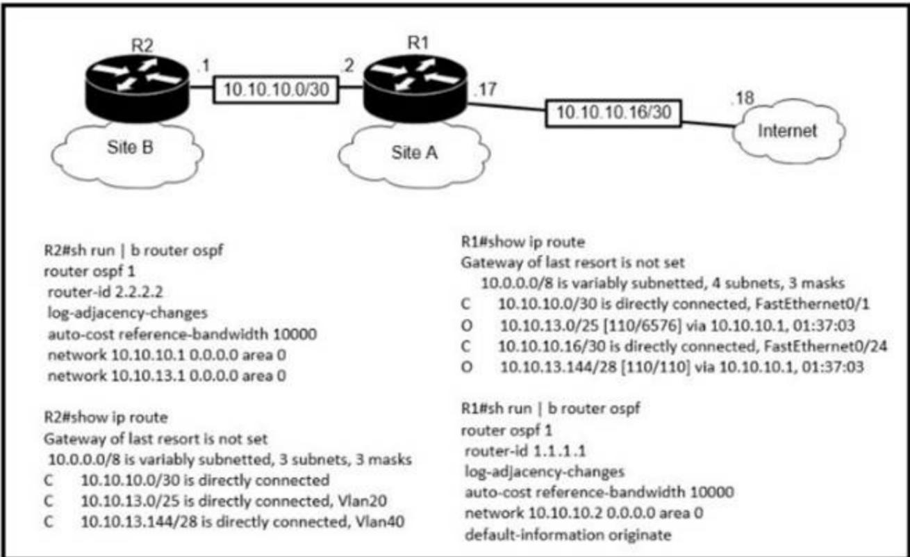
The default-information originate command is configured under the R1 OSPF configuration After testing workstations on VLAN 20 at Site B cannot reach a DNS server on the Internet Which action corrects the configuration issue?
