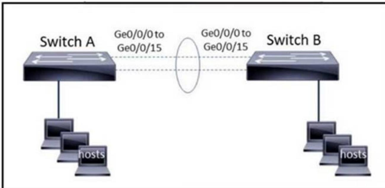
The EtherChannel is configured with a speed of 1000 and duplex as full on both ends of channel group 1. What is the next step to configure the channel on switch A to respond to but not initiate LACP communication?
