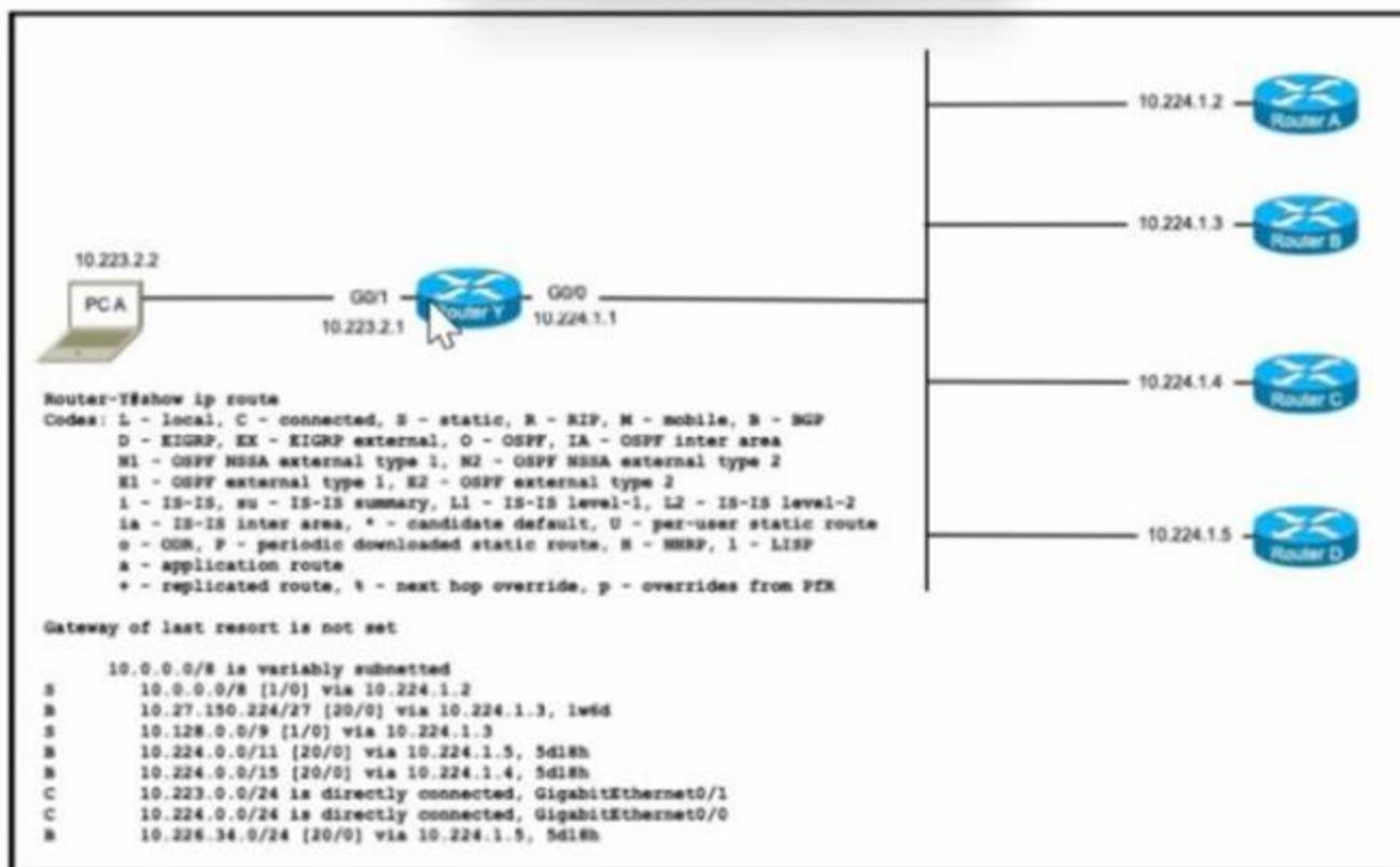
PC A is communicating with another device at IP address 10.227.225.255. Through which router does router Y route the traffic?
