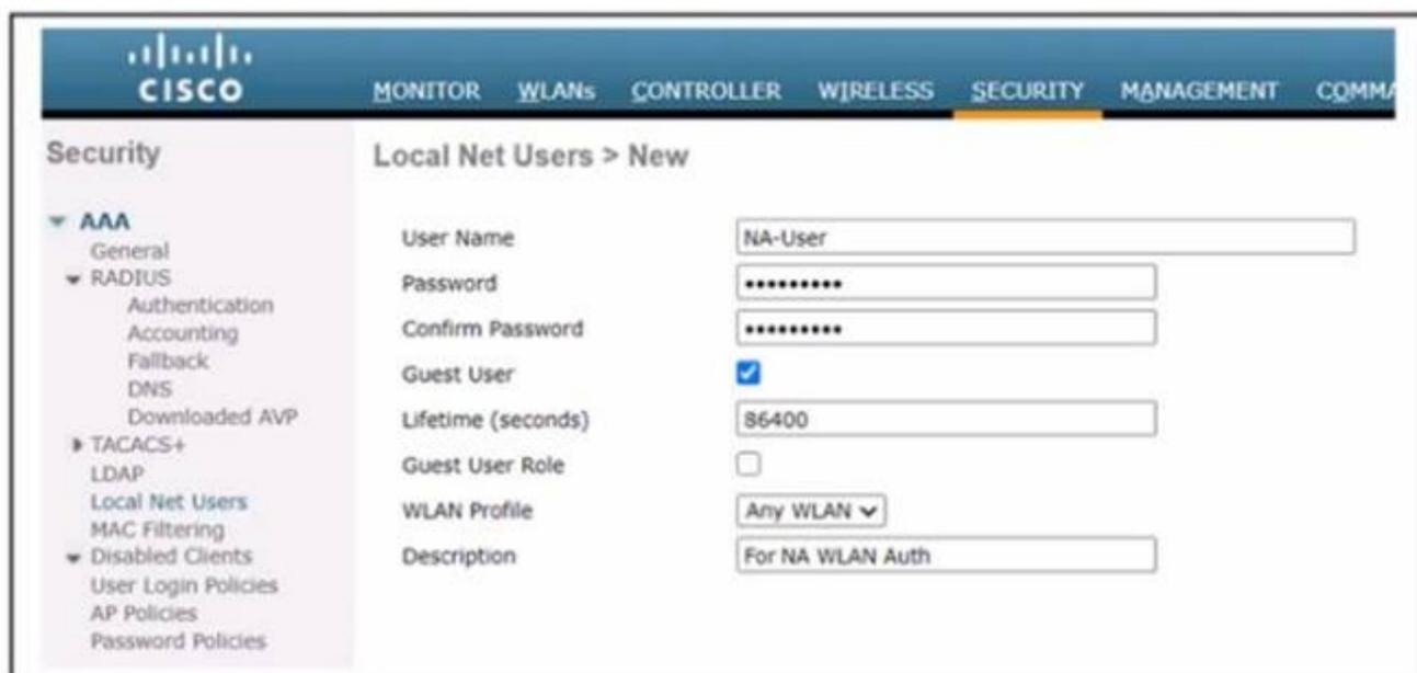
Wireless LAN access must be set up to force all clients from the NA WLAN to authenticate against the local database. The WLAN is configured for local EAP authentication. The time that users access the network must not be limited. Which action completes this configuration?
