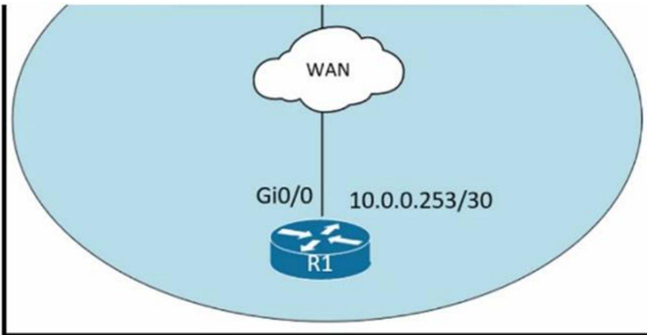
An administrator must turn off the Cisco Discovery Protocol on the port configured with address last usable address in the 10.0.0.0/30 subnet. Which command set meets the requirement?
