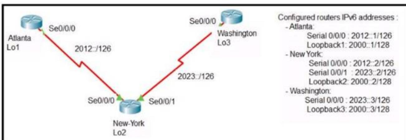
The New York router is configured with static routes pointing to the Atlanta and Washington sites. Which two tasks must be performed so that the Serial0/0/0 interfaces on the Atlanta and Washington routers can reach one another? (Choose two.)
