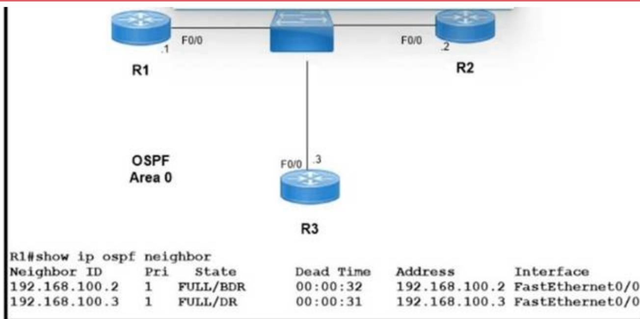
Which two configurations must the engineer apply on this network so that R1 becomes the DR? (Choose two.)
