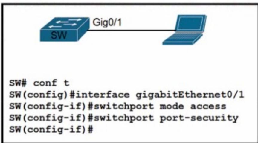
A network engineer started to configure port security on a new switch. These requirements must be met:
