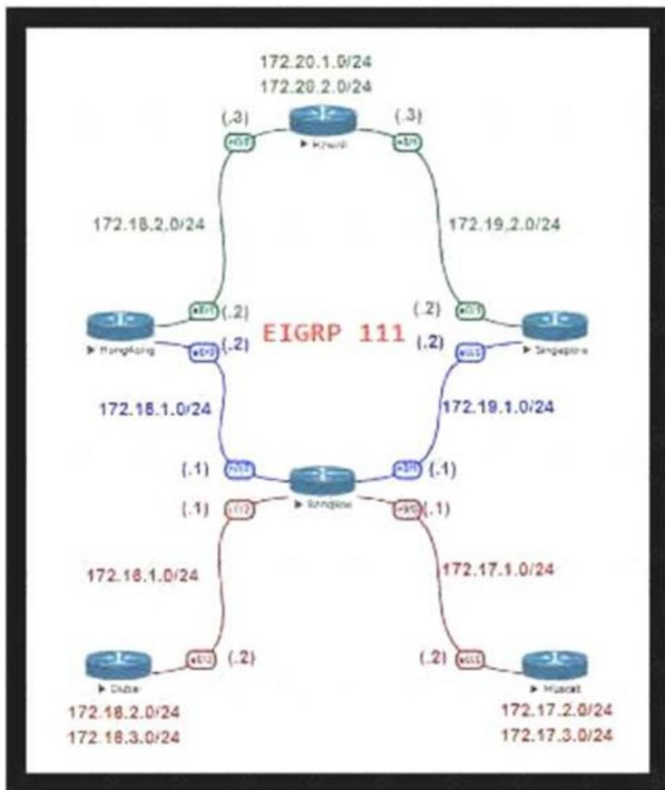
For Company XYZ Bangkok is using ECMP to reach the 172.20.2.0/24 network. The company wants a design that would allow them to forward traffic from 172.16.2.0/24 toward 172.20.2.0/24 via the Singapore router as the preferred route. The rest of the traffic should continue to use ECMP. Which technology fulfills this design requirement?
