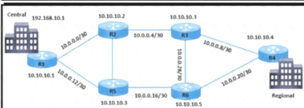
Refer to me exhibit Traffic from R3 to the central site does not use alternate paths when R3 cannot reach 10 10 10 2 Traffic on R3 destined to R4 takes an alternate route via 10 10 10.6 when 10 10 10 4 is not accessible from R3 Which configuration switches traffic destined to 10 10 10 2 from R3 on the alternate path”
