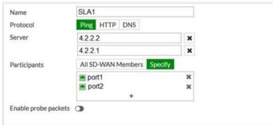
The screenshot shows the configuration for a performance SLA named 'SLA1'. The 'Protocol' is set to 'Ping'. The 'Server' field contains two entries: '4.2.2.2' and '4.2.2.1'. The 'Participants' field is set to 'All SD-WAN Members' with a 'Specify' button. Below this, two ports are listed: 'port1' and 'port2'. The 'Enable probe packets' checkbox is currently unchecked.
