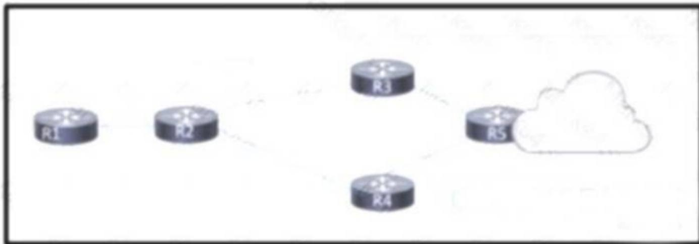
An engineer is scripting ACLs to handle traffic on the given network. The engineer must block users on the network between R1 and R2 from leaving the network through R5. but these users must still be able to access all resources within the administrative domain. How must the engineer implement the ACL configuration?
