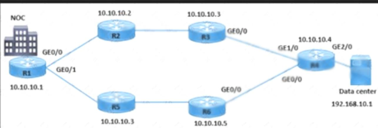
Refer to the exhibit An enterprise operations team must monitor all application server traffic in the data center The team finds that traffic coming from the hub site from R3 and R6 rs monitored successfully but traffic destined to the application server is not monitored Which action resolves the issue?
